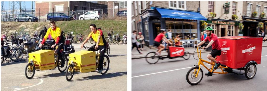
Fig. 3-2. Examples of 2-wheel cargo bikes as used by DHL and a 3-wheel tricycle as used by Outspoken Delivery. Photo credit: Mark Wagenbuur and Outspoken Delivery.
