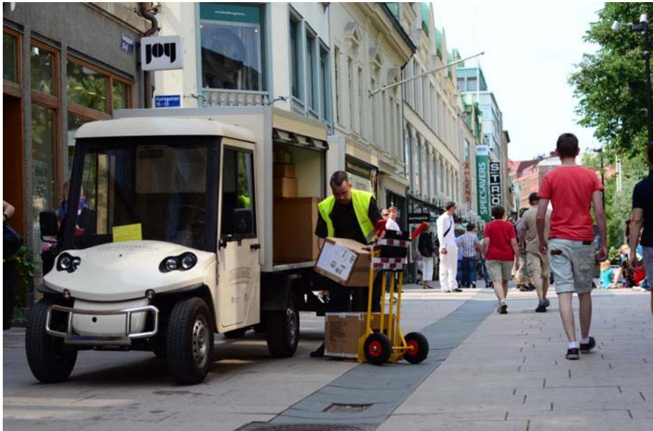
The Melex 390 with custom trailer has a 5000 watt motor and a total cargo capacity of 2000 kg and 6 m<sup>3</sup>. Energy consumption: 1,8 kWh/10 km. Width: 125 cm.
