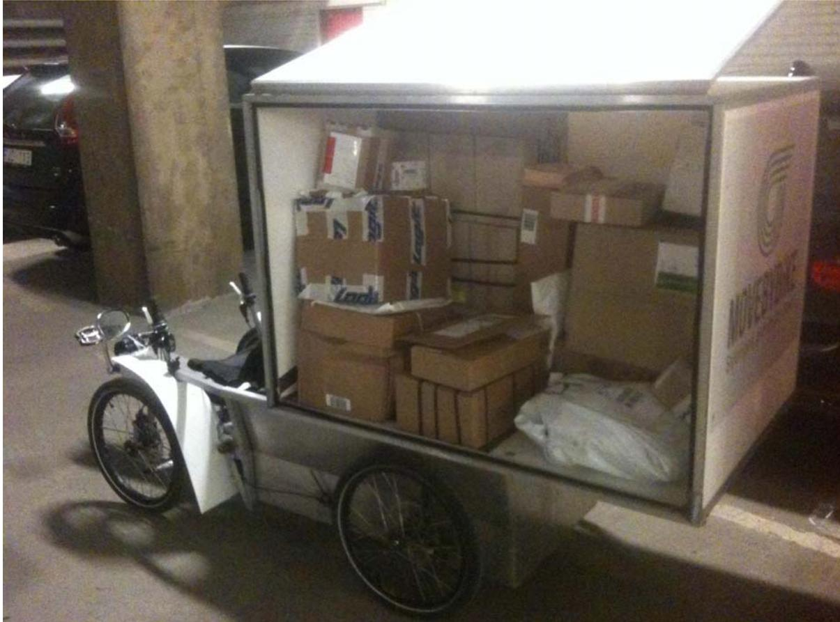
The Velove cargobike prototype has four wheels and is equipped with a 250 watt Sunstar iBike crank assist. It has a 0,9 m<sup>3</sup> weatherproof and lockable cargobox. Energy consumption: appr. 0.2 kWh/10 km. Width: 87 centimeters.
