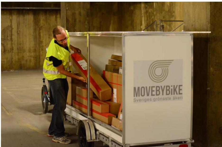
The Nihola is equipped with a 250 watt 8fun assist. The trailer from Bikes at Work has a 280 kg capacity, but we do not load it to more than 150 kg due to that Gothenburg is a hilly city. The trailer has a 2.3 m<sup>3</sup> weatherproof and lockable cargobox from Velove. Energy consumption: appr. 0,4 kWh/10 km. Trailer width: 109 centimeters.
